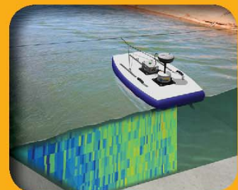
3-D velocity profiling, bathymetric measurement and discharge calculation as you transect a channel.
